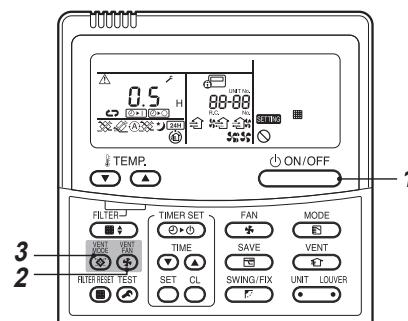
**1 Push the
