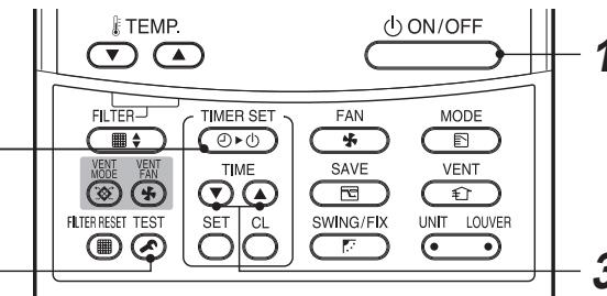
1 Push the
